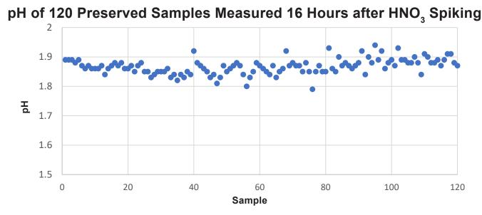
After automated preservation using **TRAX**Station, 120 samples were held for 16 hours before pH measurement. These data show that the pH values for all samples were less than 2 (average pH = 1.86 with an RSD of 1.39%), proving that **TRAX**Station effectively preserves water samples as described in EPA Method 200.2, Section 8.1.
