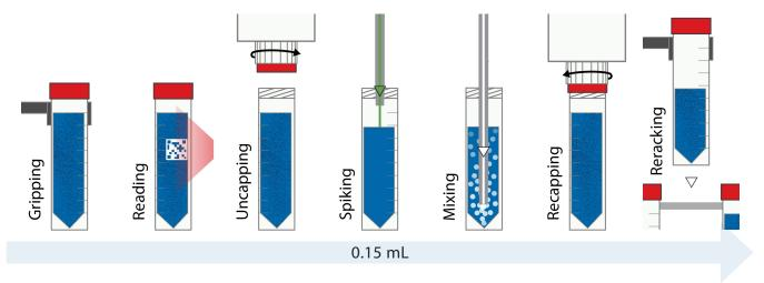
TRAXStation automatically and completely prepares racked samples for preservation. LuerProbe is used for spiking and mixing steps. Other probe options are available.
